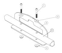
In the bag of parts for the lifting eye, ensure all of the required materials are included: 2 qty - 5/16-18 x 2.25 button head socket screws (#1); 2 qty - washers (#2); 2 qty - .3125-18 flange (#3); 1 qty - lifting eye (#4).
