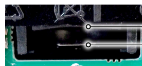
Install Battery Between These Two Points
