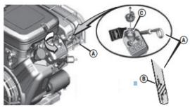
Oil is added to the engine by removing the oil cap and adding oil at this point. After filling the crankcase to the proper level, be sure you properly tighten the oil fill cap ('C').
