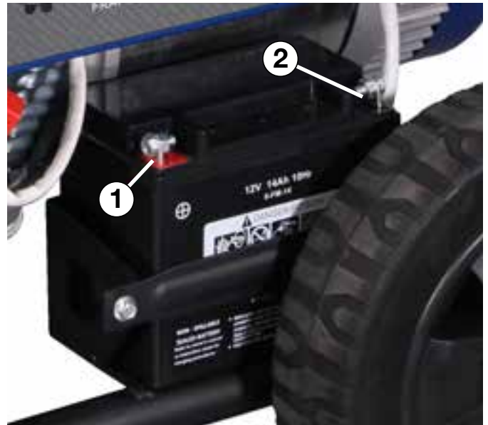
Figure 6 - Attaching the Negative (-) Battery Wire (black)
