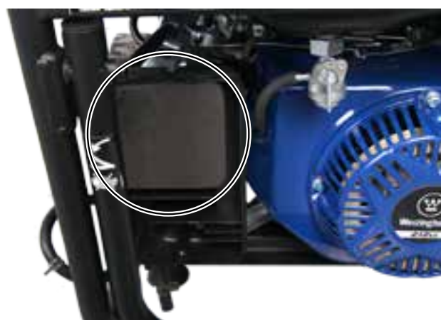
Figure 30 - Remove Coarse Air Filters
