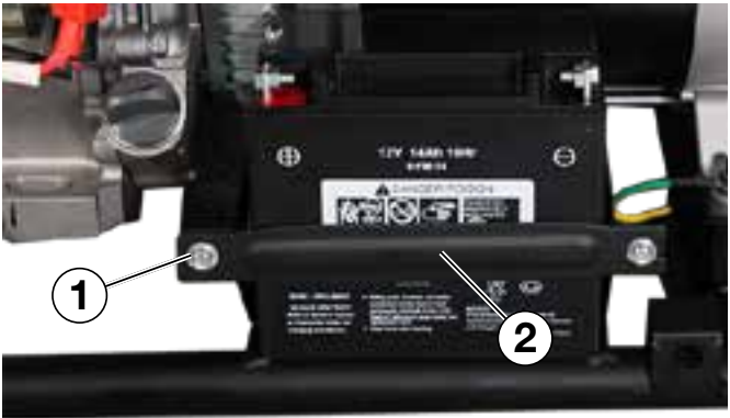
Figure 36 - (1) Bolt, (2) Battery Hold Down Plate
