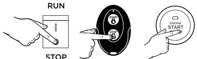
Figure 13 - Stopping the generator
