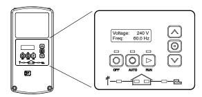
The RDC2 controller provides integrated control for the generator set, Kohler® Model RXT transfer switch, programmable interface module (PIM), and load management device.
