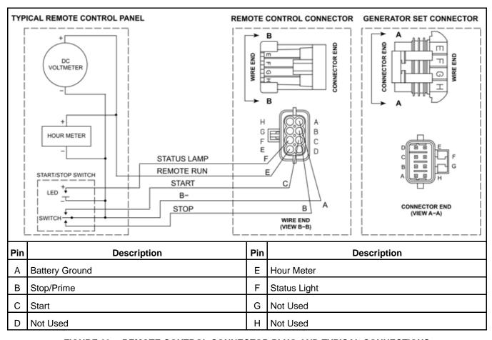
FIGURE 29. REMOTE CONTROL CONNECTOR PLUG AND TYPICAL CONNECTIONS
