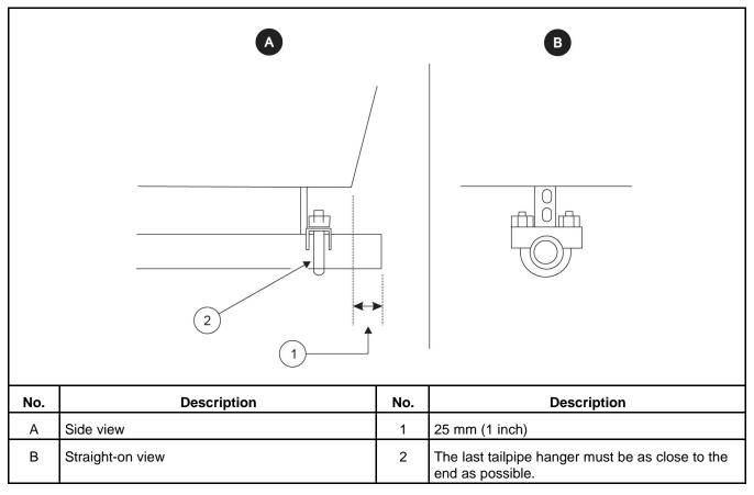
FIGURE 11. TERMINATING THE EXHAUST TAILPIPE
