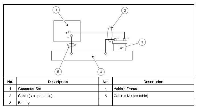
FIGURE 31. VEHICLE FRAME AS PATH FROM BATTERY NEGATIVE (-) TERMINAL
