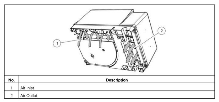
FIGURE 4. GENERATOR SET COOLING AIR INLET AND OUTLET
