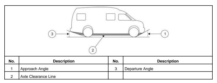
FIGURE 13. VEHICLE CLEARANCES - CLASS B VAN
