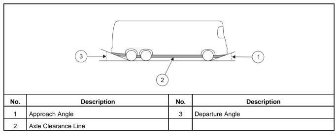
FIGURE 12. VEHICLE CLEARANCES - CLASS A RV
