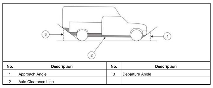
FIGURE 14. VEHICLE CLEARANCES - PICKUP TRUCK CAMPER
