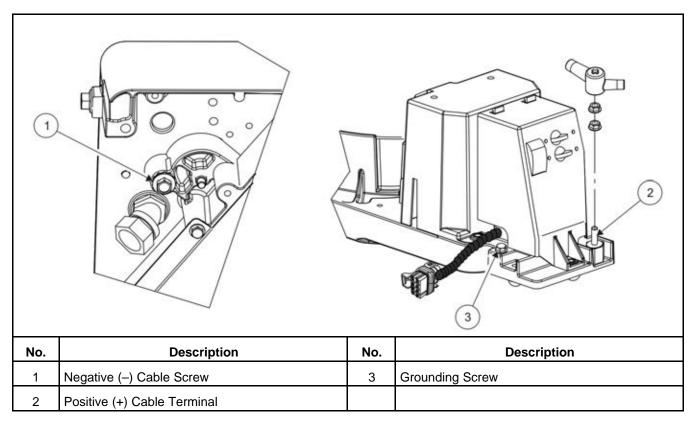
FIGURE 32. BATTERY CABLE CONNECTIONS
