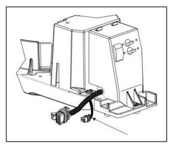
FIGURE 22. REMOTE PUMP WIRING CONNECTOR
