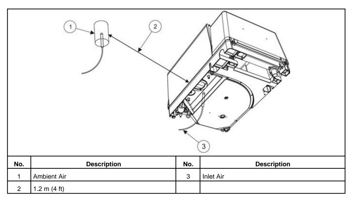
FIGURE 33. THERMOCOUPLE LOCATIONS FOR HOT AIR RECIRCULATION TEST
