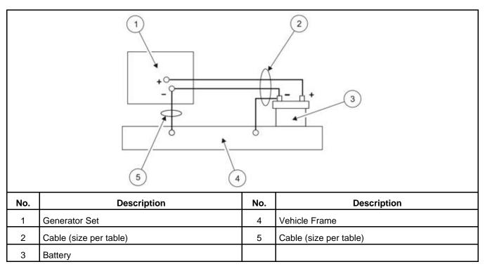
FIGURE 30. FULL-LENGTH CABLE FROM BATTERY NEGATIVE (-) TERMINAL
