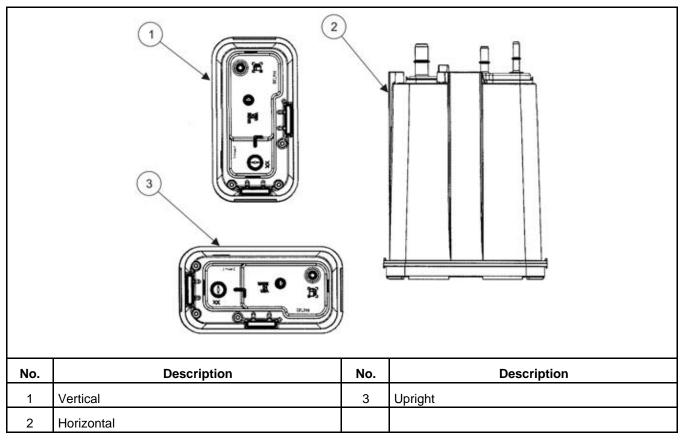
FIGURE 18. ACCEPTABLE CANISTER MOUNTING ORIENTATIONS
