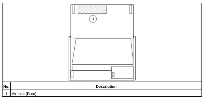
FIGURE 7. SIDE AIR INTAKE AND BOTTOM AIR DISCHARGE
