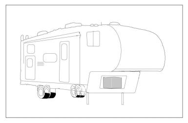
FIGURE 3. TYPICAL GENERATOR SET LOCATIONS - 5TH WHEEL RV
