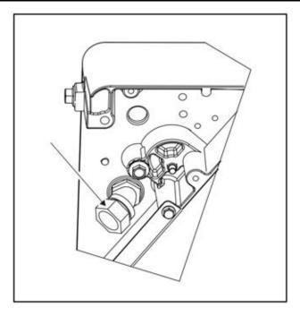
FIGURE 26. AC OUTPUT CONDUIT
