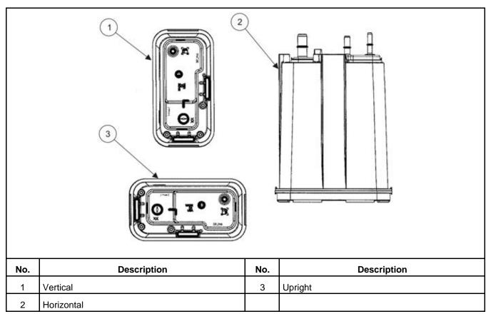
FIGURE 20. ACCEPTABLE CANISTER MOUNTING ORIENTATIONS
