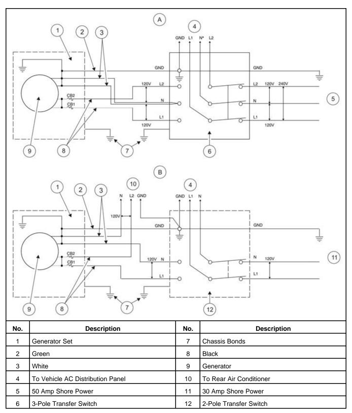
FIGURE 27. TYPICAL CONNECTIONS WITH TRANSFER SWITCH AND UTILITY
