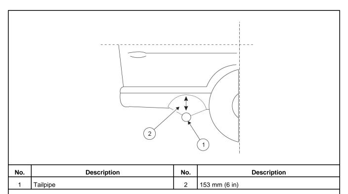
No opening into the vehicle interior may be closer than 153 mm (6 in) to the end of the tail pipe (within area 2, identified in this image).
