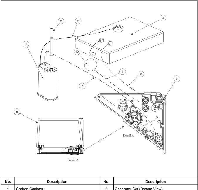
1 Carbon Canister 6 Generator Set (Bottom View) 2 5/8 in Vent Hose to clean outside air space or PN 7 5/16 in Purge Hose (Vapor) 0148-1343 Vent Filter 3 5/16 in Evaporative Capture Hose (vapor) 8 5/16 in Fuel Line from Pump (liquid) 9 4 Fuel Tank 1/4 in Fuel Return Line (liquid) EFI Pump 5 Generator Set (End View) 10
