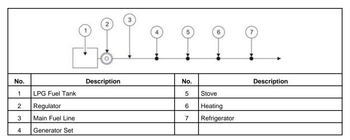
FIGURE 24. LPG FUEL LINE APPLIANCE CONNECTIONS (2.5 THROUGH 5.5 KW LPG SYSTEMS)
