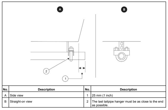
FIGURE 7. TERMINATING THE EXHAUST TAILPIPE
