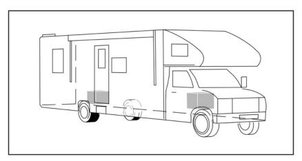
FIGURE 2. TYPICAL GENERATOR SET LOCATIONS - CLASS C RV
