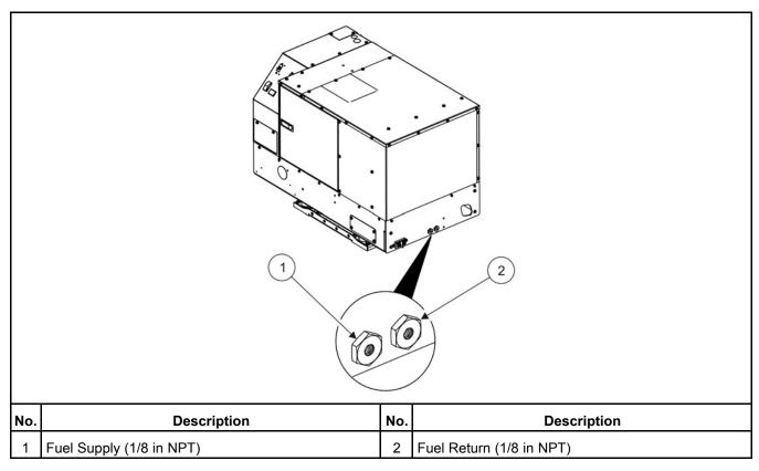
FIGURE 9. FUEL CONNECTIONS
