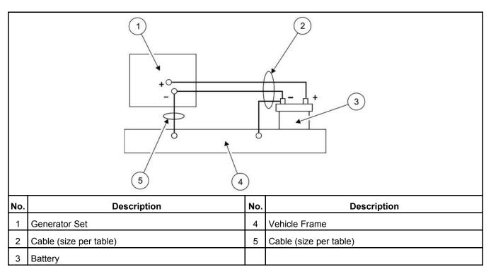
FIGURE 14. FULL-LENGTH CABLE FROM BATTERY NEGATIVE (-) TERMINAL
