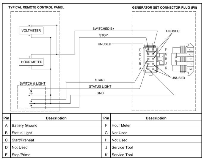
FIGURE 13. REMOTE CONTROL CONNECTOR PLUG AND TYPICAL CONNECTIONS
