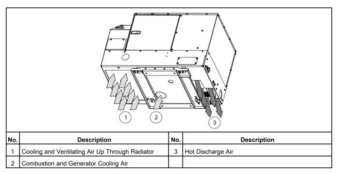
FIGURE 3. COOLING, VENTILATION, AND COMBUSTION AIR FLOWS
