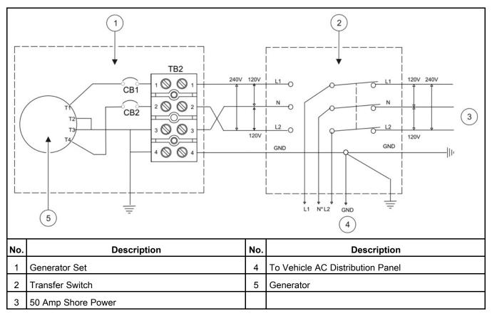
FIGURE 11. TYPICAL CONNECTIONS WITH TRANSFER SWITCH AND UTILITY
