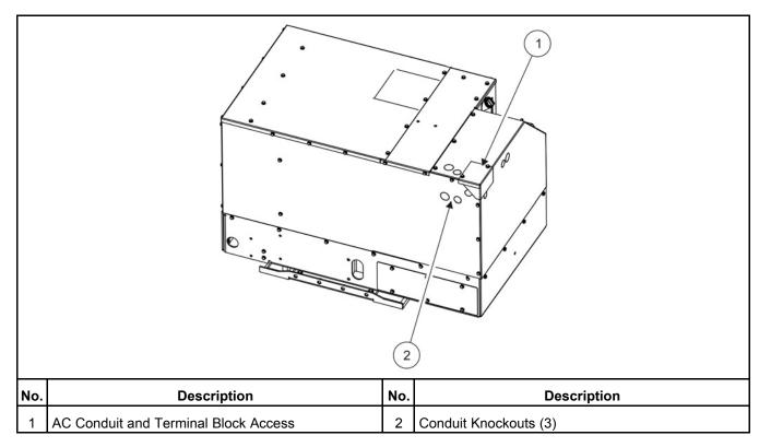
FIGURE 10. AC OUTPUT CONDUIT
