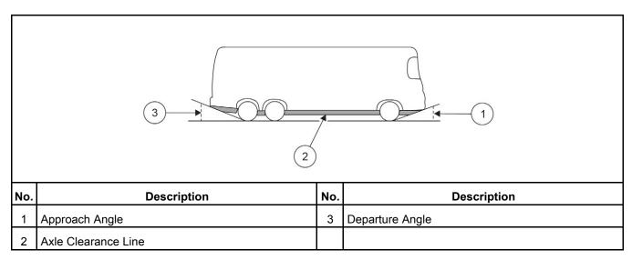
FIGURE 8. VEHICLE CLEARANCES - CLASS A RV
