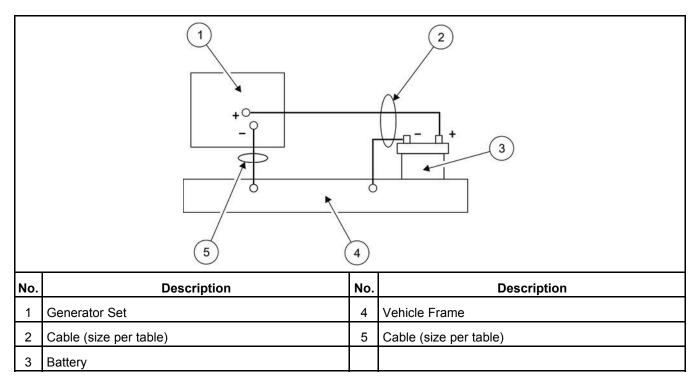
FIGURE 15. VEHICLE FRAME AS PATH FROM BATTERY NEGATIVE (-) TERMINAL
