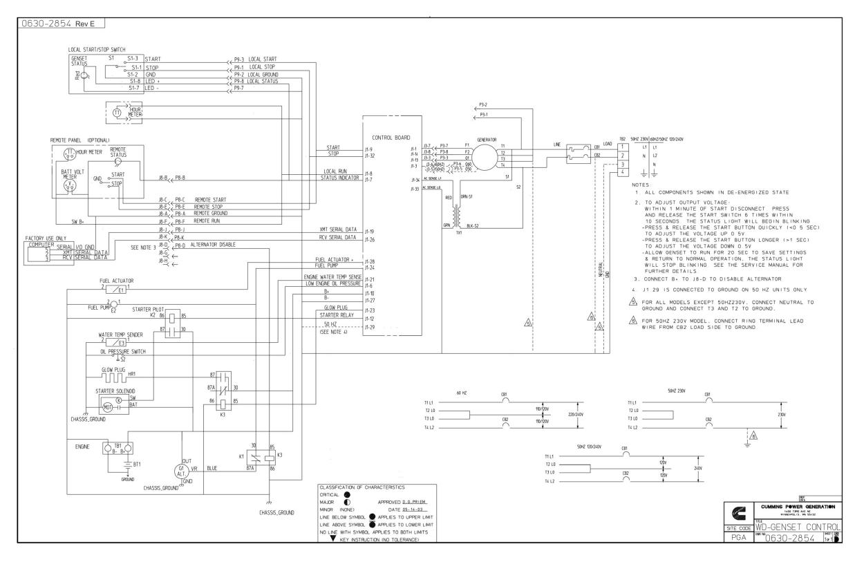
FIGURE 19. WIRING DIAGRAM GENSET CONTROL
