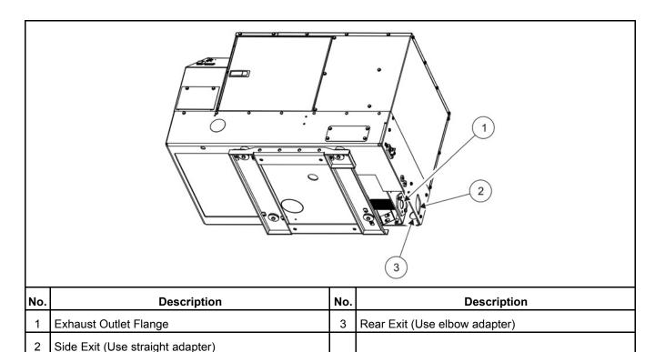
FIGURE 4. TAILPIPE INSTALLATION
