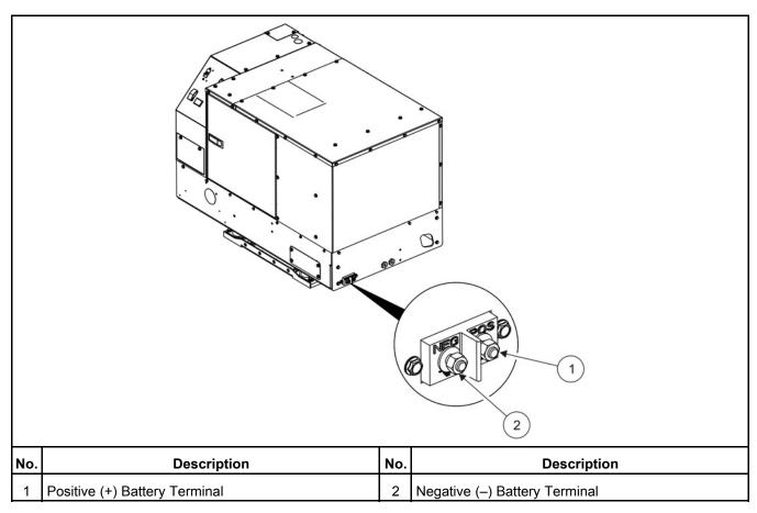
FIGURE 16. BATTERY CABLE CONNECTIONS
