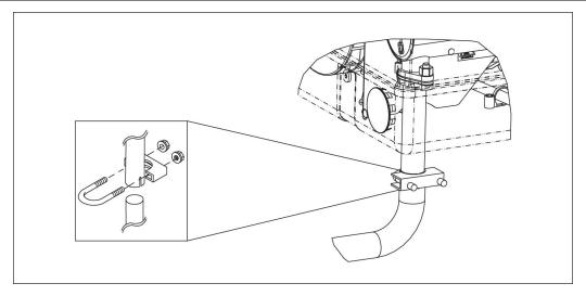
FIGURE 5. EXHAUST TAILPIPE CONNECTIONS
