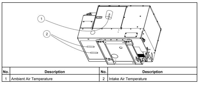
FIGURE 17. THERMOCOUPLE LOCATIONS FOR HOT AIR RECIRCULATION TEST
