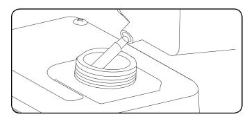
6. Screw on the fuel cap and wipe away any spilled fuel.
