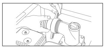
2. Slide the blue discharge hose over the discharge fitting (top of pump) and secure with the hose clamp (74-79 mm ID) with wrench.
