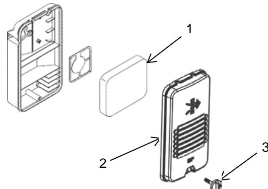
Remove the air filter cover bolt (3) and remove the air filter cover (2). Make sure that the air filter (1) is clean and not damaged. If the air filter is dirty, wash the filter. If the air filter is damaged, replace the air filter.
