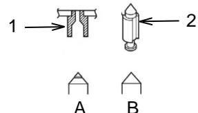
Check the float valve seat (1) and float valve (2) for wear. Figure A shows a worn float valve that needs replaced. Figure B shows a float valve that can be reused.
