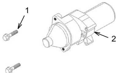
Remove starter mounting bolts (1) from the front of the crankcase and remove starter (2) from the side of the crankcase. Reinstall in reverse order.
