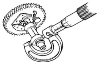
Inspect the camshaft for damage or abnormal wear. Measure the lift on the camshaft lobes. The acceptable limits for the lift are shown in the table below. If the lift is out of the acceptable range, replace the camshaft.
