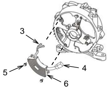
Disconnect leads (3) from the brush and unplug connector (4). Remove bolts (5) and voltage regulator (6). Reinstall in reverse order. The red lead goes onto the "+" terminal of the brush. The white lead goes onto the "-" terminal of the brush.
