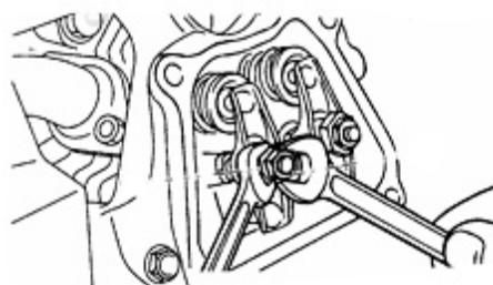
Loosen the locking nut. Turn the adjustment nut clockwise to decrease the gap. Turn the adjustment nut counterclockwise to increase the gap. When the valve clearance is within tolerance, tighten the locking nut to  $8\pm1$  N·m ( $6\pm1$  lb ft). Reinstall the valve cover gasket and valve cover. Check the spark plug washer to
