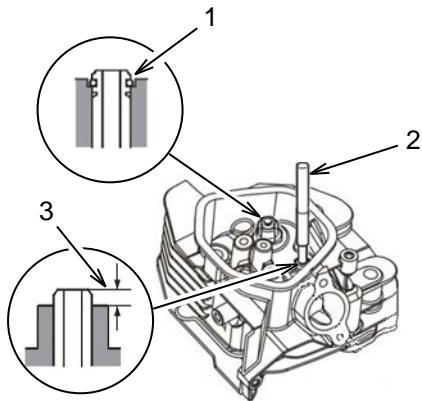
Install the new valve guides from the valve spring side of the cylinder head. Use the valve guide driver (2) to drive the exhaust valve guide in until the clip is fully seated (1). Drive the intake valve guide in until the top of the valve guide extends 1mm above the cylinder head (3). After installation check each valve guide for damage. If damaged, repeat the removal and installation process using a new valve guide.
