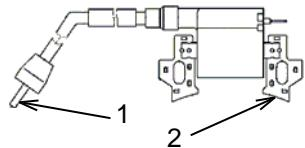
Measure the resistance of the secondary coil by touching one lead of an Ohmmeter to the spark plug wire (1) and touching the other lead to the metal frame (2). For the RP5500 the resistance should be from 5.6 – 6.6kΩ. For the RP6500E and RP7500E the resistance should be from 5.9 – 7.1kΩ. If the resistance is not within the proper range, replace the coil.
