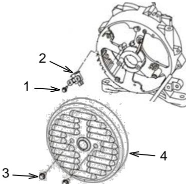
Remove bolts (3) and remove motor cover (4).
