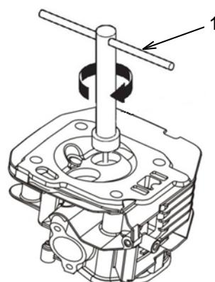
If the marking compound shows that the valve seat is not concentric, use a 45° valve seat cutter (1) to produce a smooth, concentric seat. Always turn the cutter clockwise. Use both the
