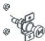
The choke control is held to the rear of the panel with 7mm nuts. Remove the choke knob and cable from the front of the panel, and remove the nuts that hold the choke to the panel. Remove the choke control from the rear of the panel. Reinstall in reverse order.
