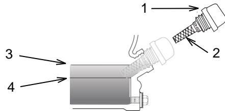
1. Remove the oil filler cap (1) and wipe the oil level gauge (2) to clean it.
