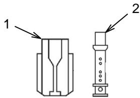
Inspect main fuel jet (1) and main fuel nozzle (2). If worn, replace.
