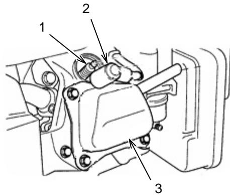
Remove spark plug cap (2), spark plug (1), valve cover (3), and valve cover gasket. Lightly pull the recoil starter until the piston is at top dead center.
