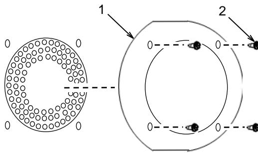
Remove screws (2). Remove spark arrestor (1). Check the spark arrestor. Carefully clean the spark arrestor with a soft wire brush. If the spark arrestor is damaged, replace the spark arrestor.
