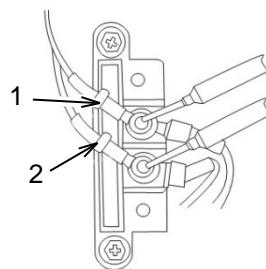
On the terminal block, use an Ohmmeter or multimeter to measure the resistance of the main winding. Place the meter across the white wire (1) and the brown wire (2). The resistance should be  $0.35\Omega \pm 10\%$  at  $25^\circ\text{C}$ . If the resistance is out of tolerance, replace the generator. Measure the resistance from the wires to ground. The resistance should be infinite. If the resistance is not infinite, replace the generator.
