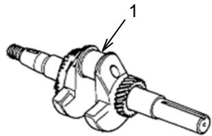
Check the diameter of the crankshaft journal (1). A normal diameter is 29.975-29.991mm. If the diameter is 29.92mm or less, replace the crankshaft.
