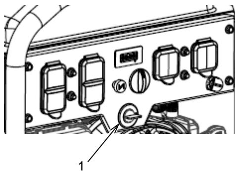
The fuel valve (1) can be accessed without removing the control panel. To remove the fuel valve, drain the fuel from the fuel tank into an appropriate container. Start the engine and let the engine run out of fuel. Turn the generator switch to the off "0" position.
