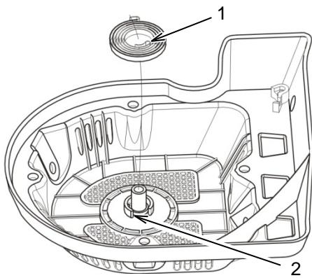
Place the inside hook (1) of the recoil starter spring in the groove (2) of the recoil starter case and set the recoil starter spring into the case. Hold the spring in place.
