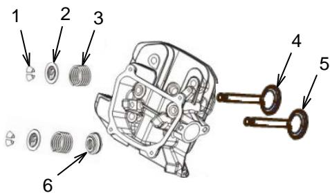
**Note:** Do not remove the retainers (2) while the head is still on the engine or the valves will drop down into the cylinder.
