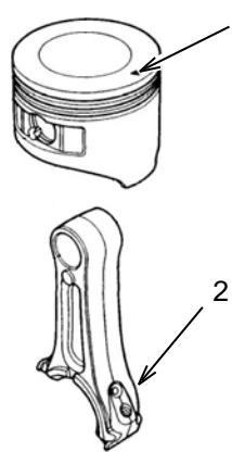
Place the connecting rod into the piston so that the longer side of the rod (2) is aligned with the mark on the piston head (1). Insert through one side of the piston, through the connecting rod, and then through the other side of the piston.
