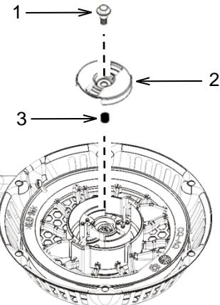
Install spring (3), drive guide (2), and fixing screw (1). Tighten the fixing screw to  $9\pm1$  N·m (6-7 lb ft).
