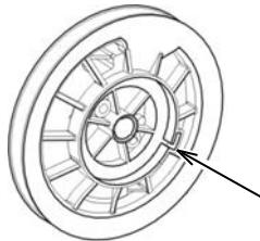
Place the outside hook of the recoil starter spring in the groove of the recoil starter pulley and hold the pulley in place.
