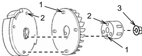
Align the positioning pins (1) on the starter cup and both sides of the impellor with the holes (2) in the starter cup and flywheel. Place the assembly on the crankshaft. Secure the assembly to the crankshaft with nut (3). Tighten the nut to  $95 \pm 4$  N·m ( $70 \pm 3$  lbft).
