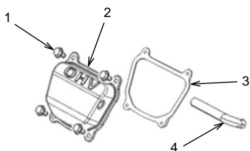
Remove valve cover bolts (1), breather tube (4), valve cover (2), and valve cover gasket (3).
