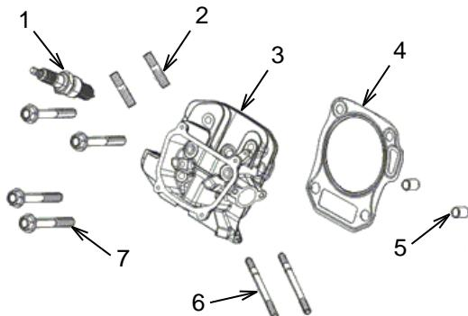
Remove spark plug (1). Remove cylinder head bolts (7), and remove cylinder head (3). Remove cylinder head gasket (4) and discard used gasket. Remove locating pins (5) and set aside. Studs (2) and (6) can remain in the cylinder head for this procedure.
