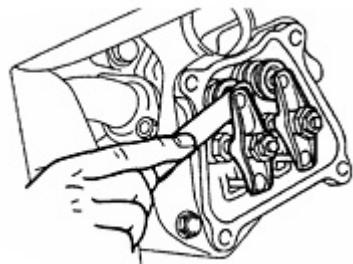
Measure the valve clearance with a feeler gauge. Refer to the following chart.
