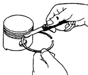
Measure the ring clearance, as shown. Normal clearance for the RP5500 is between 0.015 – 0.045mm. Normal clearance for the RP6500E and RP7500E is between 0.030 and 0.060mm. If the clearance is 0.15mm or more, replace the piston.
