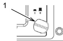
The panel light (1) is held to the panel with hot melt glue. Disconnect the panel light from the wiring and remove the glue. Remove the panel light from the front of the panel.
