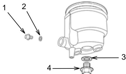
Install drain plug (1) and gasket (2) into the float chamber. Set the float chamber in place so that the drain bolt can be accessed from outside the unit. Install gasket (3) and bolt (4) to hold the float chamber in place.
