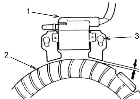
Use a feeler gauge to measure the clearance between the ignition coil (1) and the flywheel (2). For the RP5500 the clearance should be 0.2 – 0.6mm. For the RP6500E and RP7500E the clearance should be 0.4 – 0.6mm. If the clearance is out of the acceptable range, loosen screws (3) and adjust the coil so that the clearance is within range. Retighten the screws.
