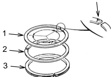
The piston rings have a mark next to the gap. Use a ring puller to install the rings with the mark facing toward the top of the piston. Make sure that you install the rings in the proper grooves, with the oil ring (3) in the lowest groove, the second ring (2) in the middle groove, and the top
