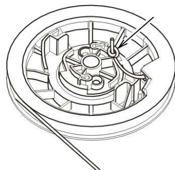
Pass the recoil starter cord through the hole in the recoil starter pulley and make a knot at the rope end as shown above.
