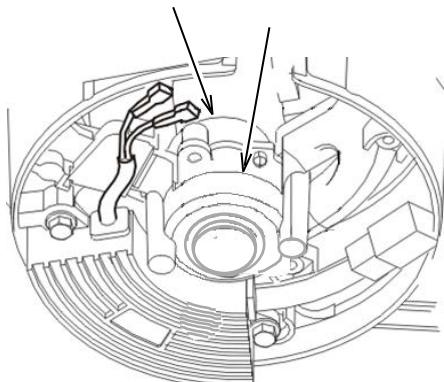
Remove the brush. Use an Ohmmeter or multimeter to measure the resistance of the collector ring at the points shown. The resistance should be  $58.5\Omega \pm 10\%$  at  $25^\circ\text{C}$ . If the resistance is out of tolerance, clean the collector ring and retest. Replace the generator if necessary.
