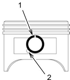
Install the piston pin clip (1) into the groove in the side of the piston. Use long nosed pliers to rotate the clip in. Do not align the gap with the cutout (2). Repeat for the other side.
