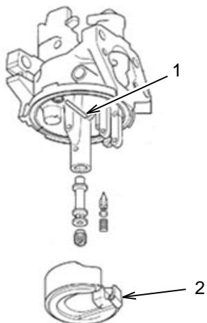
Remove float pin (1), carefully remove float (2) and contain the small parts. Clean the internal parts with carburetor cleaner and compressed air.
