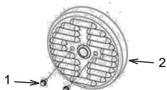
Remove bolts (1) and remove motor cover (2).
