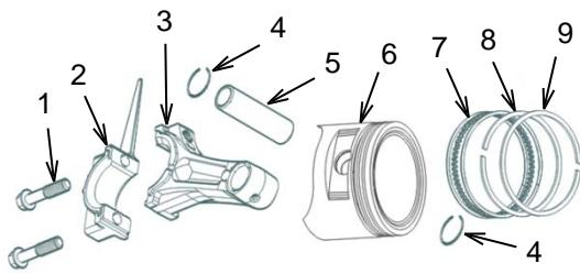
Remove the connecting rod bolts (1) and the rod cap (2). Push the connecting rod and piston out of the block. Remove any carbon deposits. Inspect the cylinder bore. If the cylinder wall is damaged, replace the crankcase. Use a ring puller to remove piston rings (7), (8), and (9).
