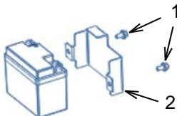
Disconnect the negative battery cable from the battery and secure it so that it will not contact the battery. Disconnect the positive battery cable. Use a Voltmeter or a multimeter set to VDC to measure the battery. If the battery has less than 12.4 volts, replace the battery. Remove bolts (1) and plate (2). Remove the battery and dispose of properly.
