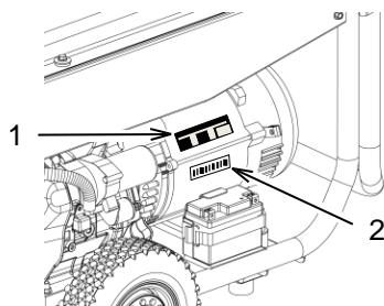
Cat portable generators are identified with model numbers, serial numbers, and with performance specification numbers. The model number and performance specifications are located on the ratings plate (1). The serial number is located on the serial number plate (2).
