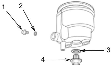
Drain the fuel from float chamber by removing drain bolt (1) and gasket (2). Use a suitable container to catch the fuel. Dispose of the fuel properly. Remove bolt (4) and gasket (3). Carefully remove the float chamber, and contain any small parts that may fall out.
