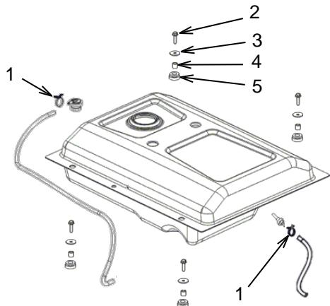
Remove hose clamps (1) and fuel lines from the rollover sensor and the fuel filter. Remove all four bolts (2), washers (3), bushings (4), and sleeves (5). Lift off the fuel tank.
