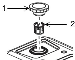
Wipe off the fuel cap (1) and surrounding area before removing the fuel cap. Wiping off the fuel cap and surrounding area before removing the fuel cap helps to reduce the amount of contaminants allowed into the fuel system.
