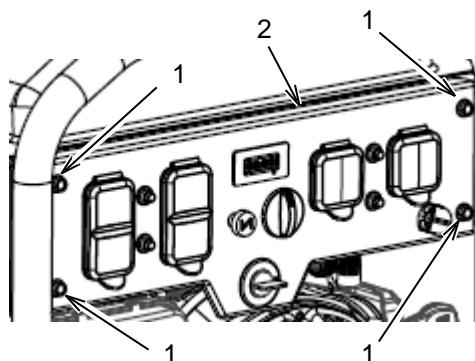
Remove bolts (1) and the washers. Pull the control panel (2) forward slowly. Make sure that the cables move freely and are not damaged. Tag the wires to identify them and then disconnect the wiring harnesses.
