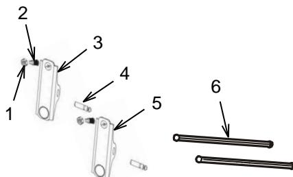
Remove locking nut (1) and adjusting nut (2). Remove pin (4), and remove exhaust valve rocker arm (3). Repeat the process for intake valve rocker arm (5). Check the rocker arms for wear. Replace if damaged. Remove pushrods (6). Inspect the pushrods. Make sure they are straight and not scored. Check the pushrod ends for wear. Replace the pushrods if worn or damaged.
