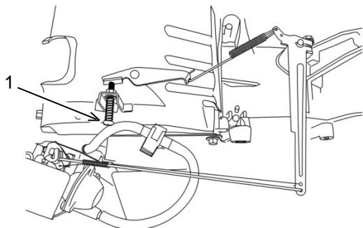
The maximum speed for this engine is 3730 – 3830 rpm. Turn the adjusting screw (1) clockwise to increase the engine speed. Turn the adjusting screw counterclockwise to decrease the engine speed.
