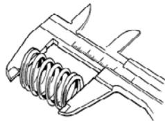
Check the free length of the valve spring. The normal free length is 37.5mm. If the free length is 37.5mm or less, replace the spring.
