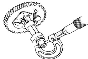
Measure the outside diameter of the camshaft. The acceptable limits for the diameter are shown in the table below. If the diameter is out of the acceptable range, replace the camshaft.
