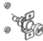
The choke control is held to the rear of the panel with nuts. Remove the choke knob and cable from the front of the panel, and remove the nuts that hold the choke to the panel. Remove the choke control from the rear of the panel. Reinstall in reverse order.
