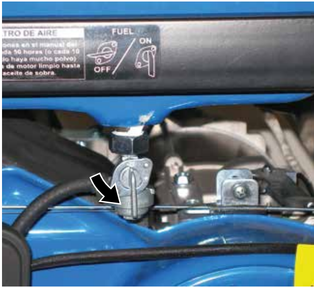
Figure 17 – Fuel Shutoff Valve in the ON Position
