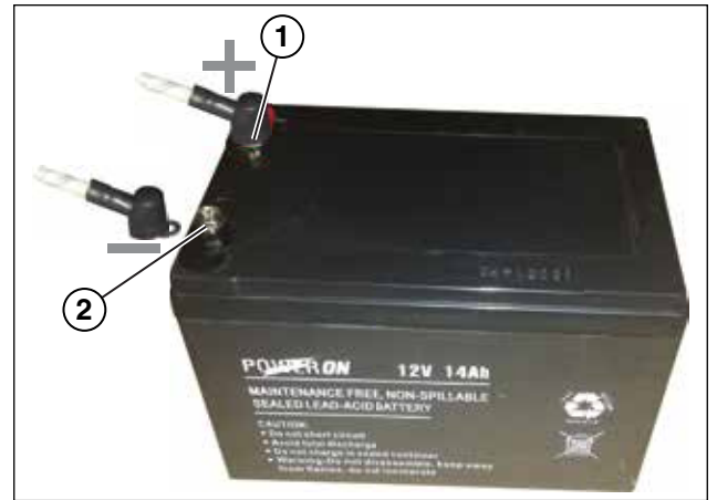
Figure 8 – Attaching the Negative (-) Battery Cable (Black)
