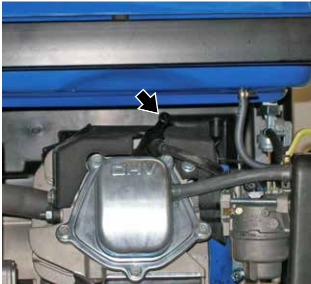
Figure 36 – Removal of Spark Plug Boot
