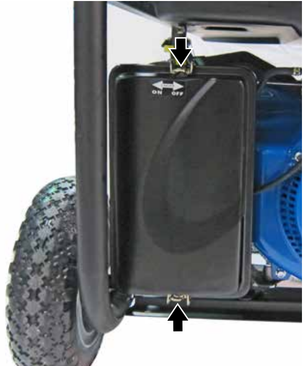
Figure 35 – Installation of Air Filter Cover
