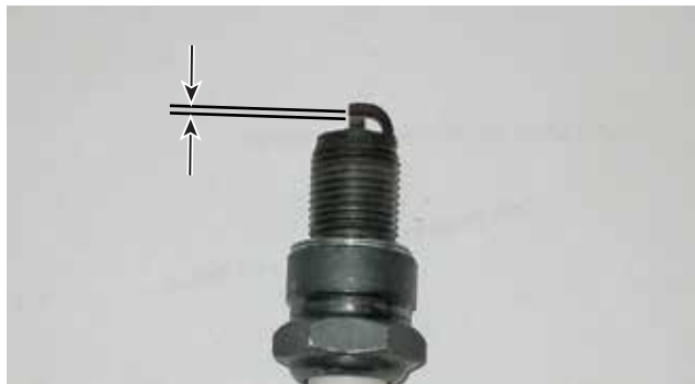
Figure 38 – Spark Plug Gap Requirements
