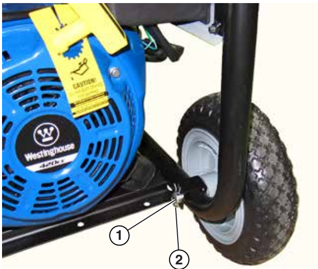
Figure 6 – Assemble Wheels to Frame
