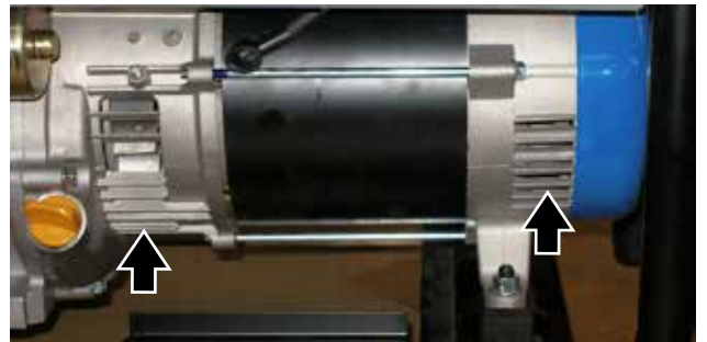
Figure 46 – Alternator Cooling Air Inlet and Outlet Port
