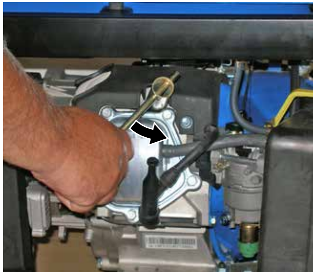
Figure 37 – Removing Spark Plug
