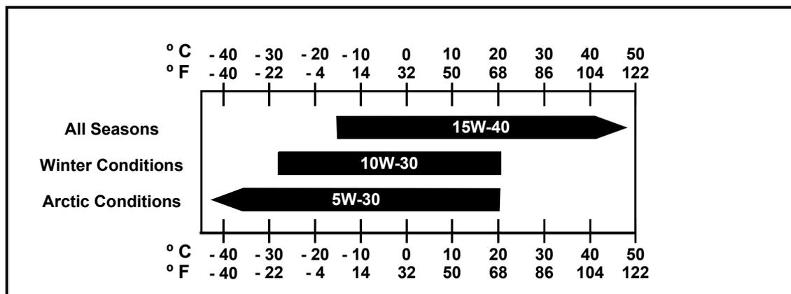
**Figure 2-2. Lubricating Oil Recommendations**
