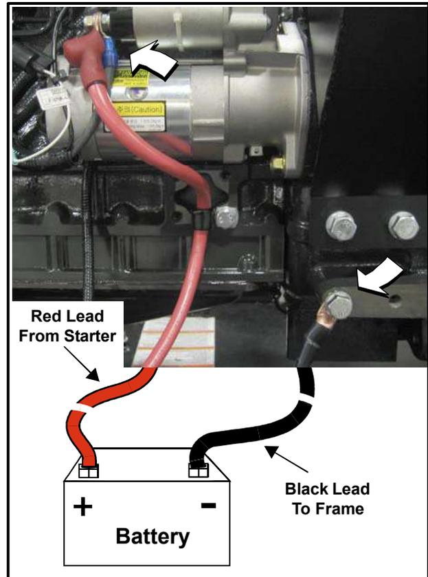
**Figure 3-4. Battery Cable Connections**
