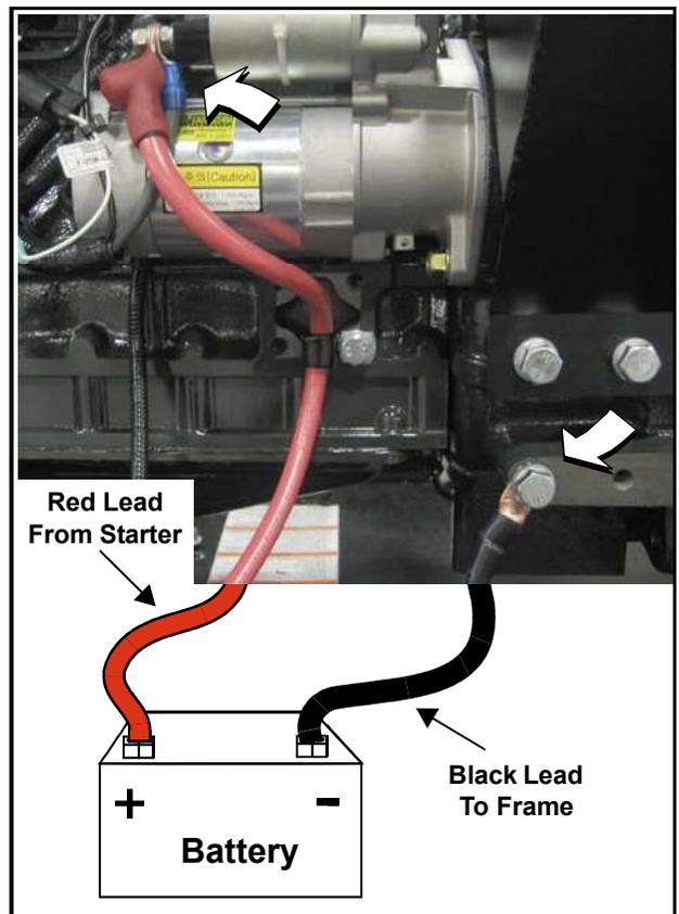
**Figure 5-11. Battery Cable Connections**
