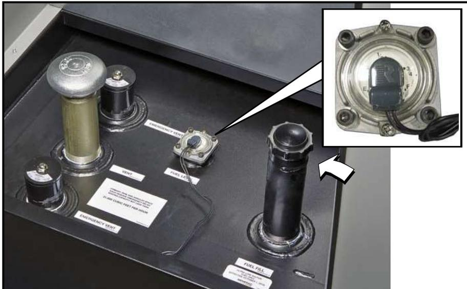
**Figure 5-7. Check Fuel Level Gauge and Fill**
