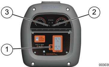
**Figure 3-5. Reset Button and Status Lights**
