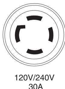
Figure 12 - 120/240 VAC, 30 Amp Receptacle
