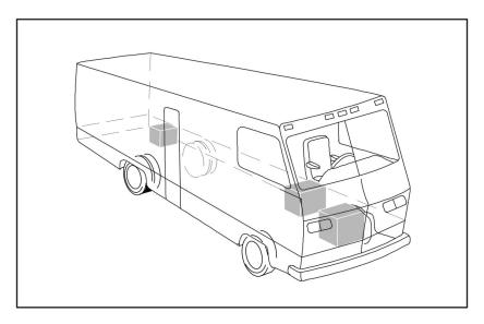
FIGURE 1. TYPICAL GENERATOR SET LOCATIONS - CLASS A RV
