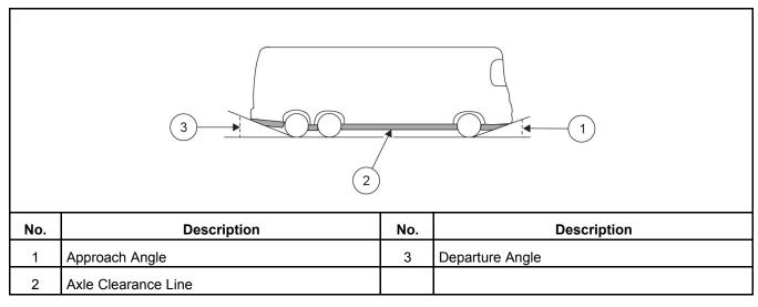
FIGURE 13. VEHICLE CLEARANCES - CLASS A RV
