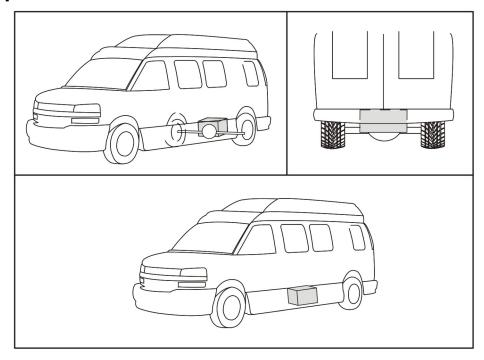
FIGURE 3. TYPICAL GENERATOR SET LOCATIONS - CLASS B VAN
