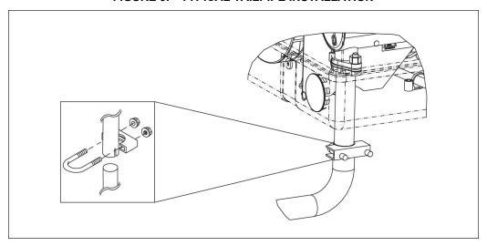
FIGURE 10. EXHAUST TAILPIPE CONNECTIONS
