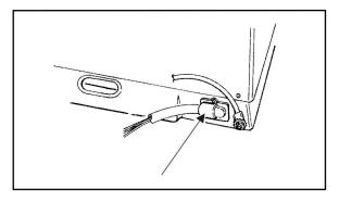
FIGURE 22. AC OUTPUT CONDUIT
