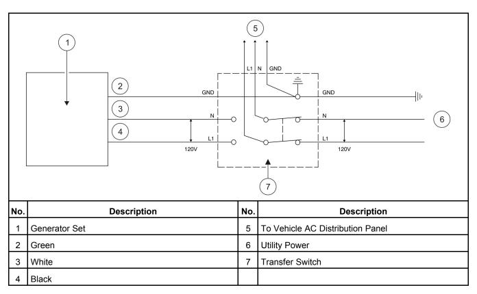
FIGURE 23. TYPICAL CONNECTIONS WITH TRANSFER SWITCH AND UTILITY
