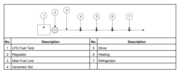
FIGURE 20. LPG FUEL LINE APPLIANCE CONNECTIONS (2.5 THROUGH 6.5 KW LPG SYSTEMS)
