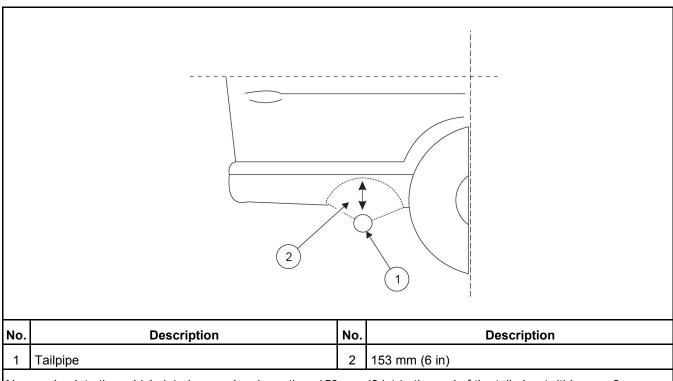
No opening into the vehicle interior may be closer than 153 mm (6 in) to the end of the tail pipe (within area 2, identified in this image).
