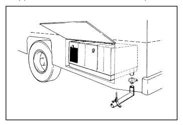
FIGURE 9. TYPICAL TAILPIPE INSTALLATION
