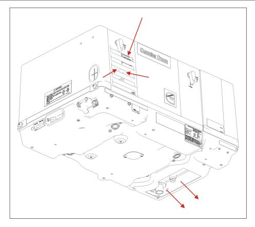
FIGURE 5. GENERATOR SET COOLING AIR INLET AND OUTLET
