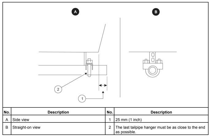
FIGURE 12. TERMINATING THE EXHAUST TAILPIPE
