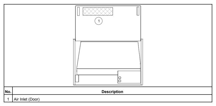
FIGURE 8. SIDE AIR INTAKE AND BOTTOM AIR DISCHARGE
