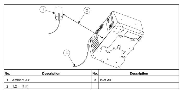
FIGURE 29. THERMOCOUPLE LOCATIONS FOR HOT AIR RECIRCULATION TEST
