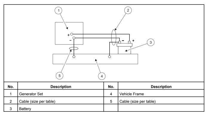
FIGURE 26. FULL-LENGTH CABLE FROM BATTERY NEGATIVE (-) TERMINAL
