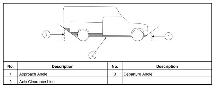
FIGURE 15. VEHICLE CLEARANCES - PICKUP TRUCK CAMPER
