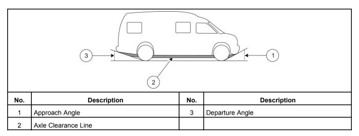
FIGURE 14. VEHICLE CLEARANCES - CLASS B VAN
