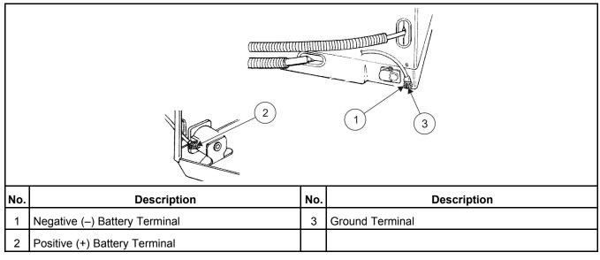
FIGURE 28. BATTERY CABLE CONNECTIONS
