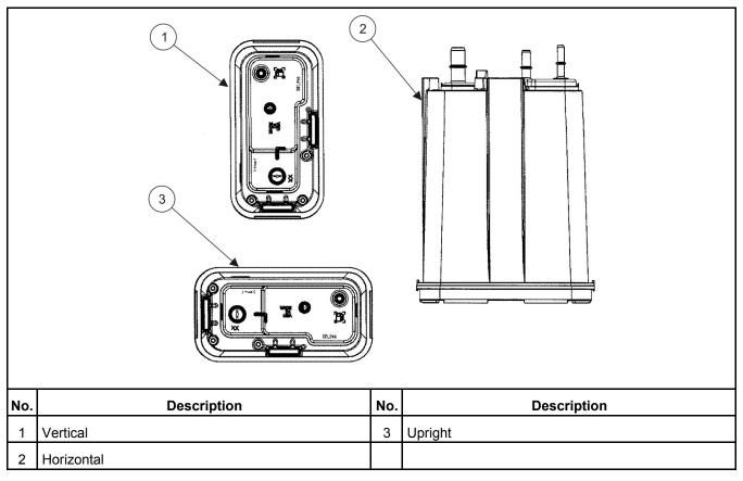
FIGURE 19. ACCEPTABLE CANISTER MOUNTING ORIENTATIONS
