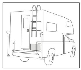
FIGURE 4. TYPICAL GENERATOR SET LOCATIONS - PICKUP TRUCK CAMPER
