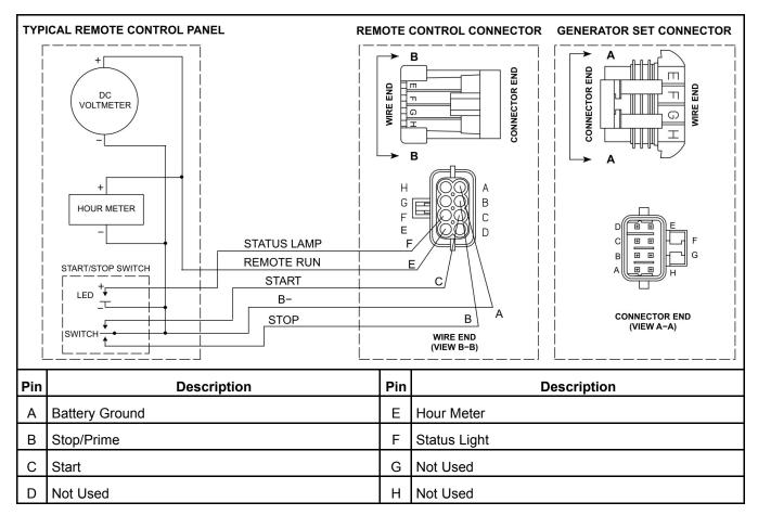
FIGURE 25. REMOTE CONTROL CONNECTOR PLUG AND TYPICAL CONNECTIONS
